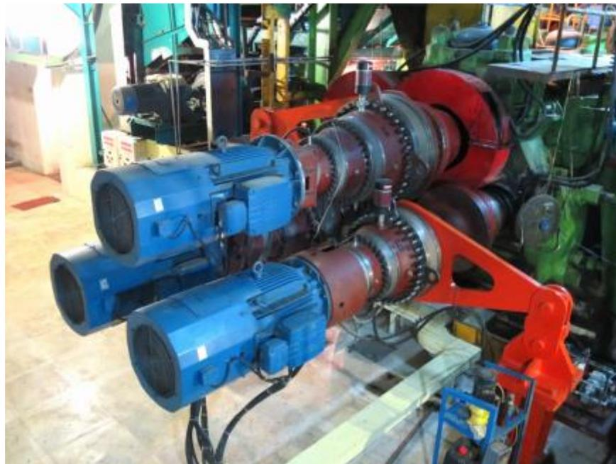
Depending on the motor size , overhung load and space constraint one other very frequent installation is a complete linear version or plano helical version as shown below
