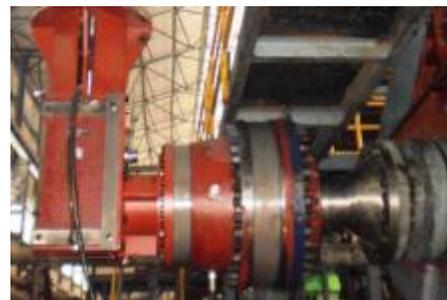
If we keep the same mounting configuration for all rollers and if the system is designed with two gearboxes on the top roller and one each on the bottom roller this gives great flexibility to mill engineer for shifting the mill rollers in tandem. This helps to reduce inventory by a huge amount as one or two sets of gearbox can be kept as spares and used among all mills depending upon number of mills.
