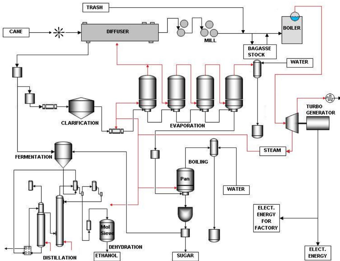
Fig. 1—Basic flow diagram of the plant.
