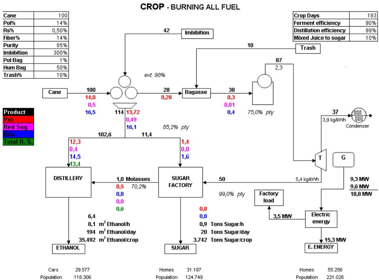
Fig. 2—Mass and energy balance of plant burning all its fuel during the crop period.
