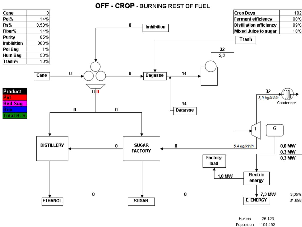
Fig. 4—Mass and energy balance of plant burning its stocked fuel during the off-crop period.
