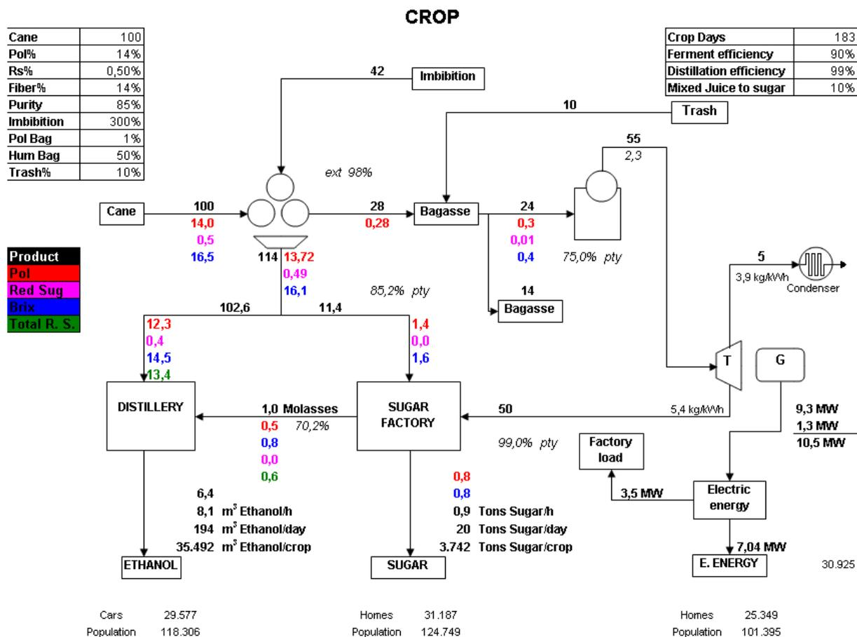
Fig. 3—Mass and energy balance of plant burning part of its fuel during the crop period.
