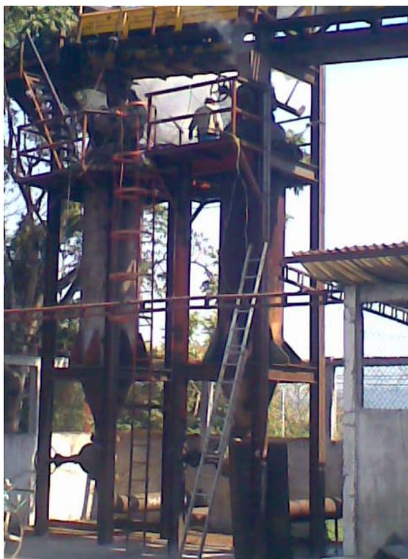
Fig. 2—Bagasse hydrolysed reactors.
