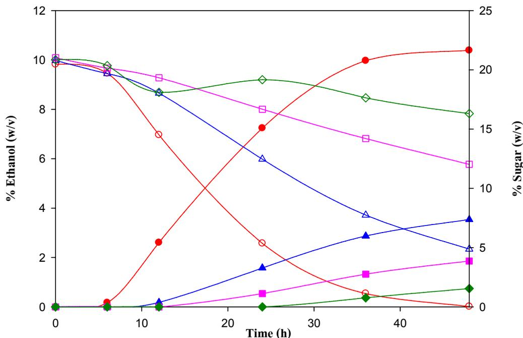
Fig. 1—Changes of ethanol and sucrose concentrations during fermentation of sucrose (20% w/v) having different calcium concentrations (0–2.16% w/v of Ca<sup>2+</sup>) by *Saccharomyces cerevisiae*. (Open symbols represent sugar contents and filled symbols represent ethanol content at different calcium concentrations; ○, ● 0%; △, ▲ 0.72%; □, ■ 1.44% and ◇, ◆ 2.16% Ca<sup>2+</sup>).
