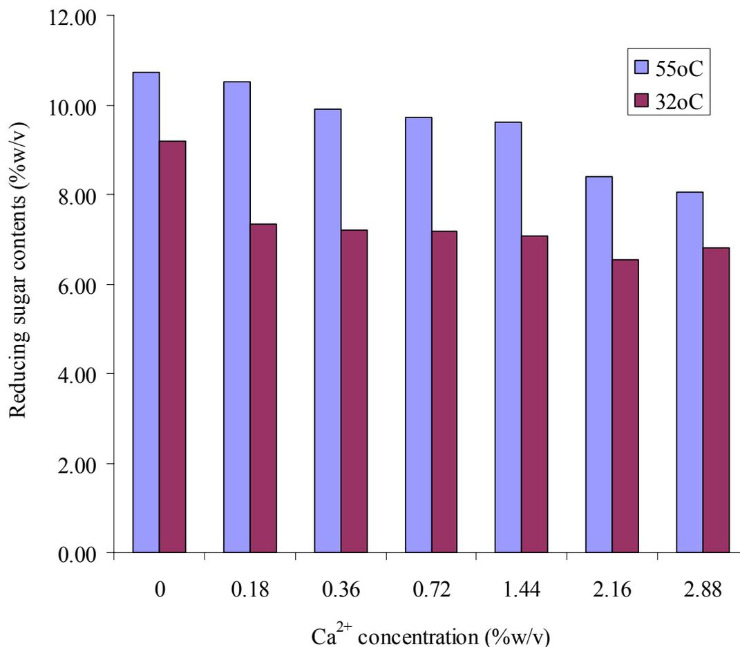
Fig. 2—Effect of calcium ( $\text{Ca}^{2+}$ ) on the hydrolytic activity of invertase enzymes (5.84 mg/mL at pH 4.5) when incubated with sucrose solutions (10% w/v) containing different calcium concentrations at 32 and 55°C for 1 h.
