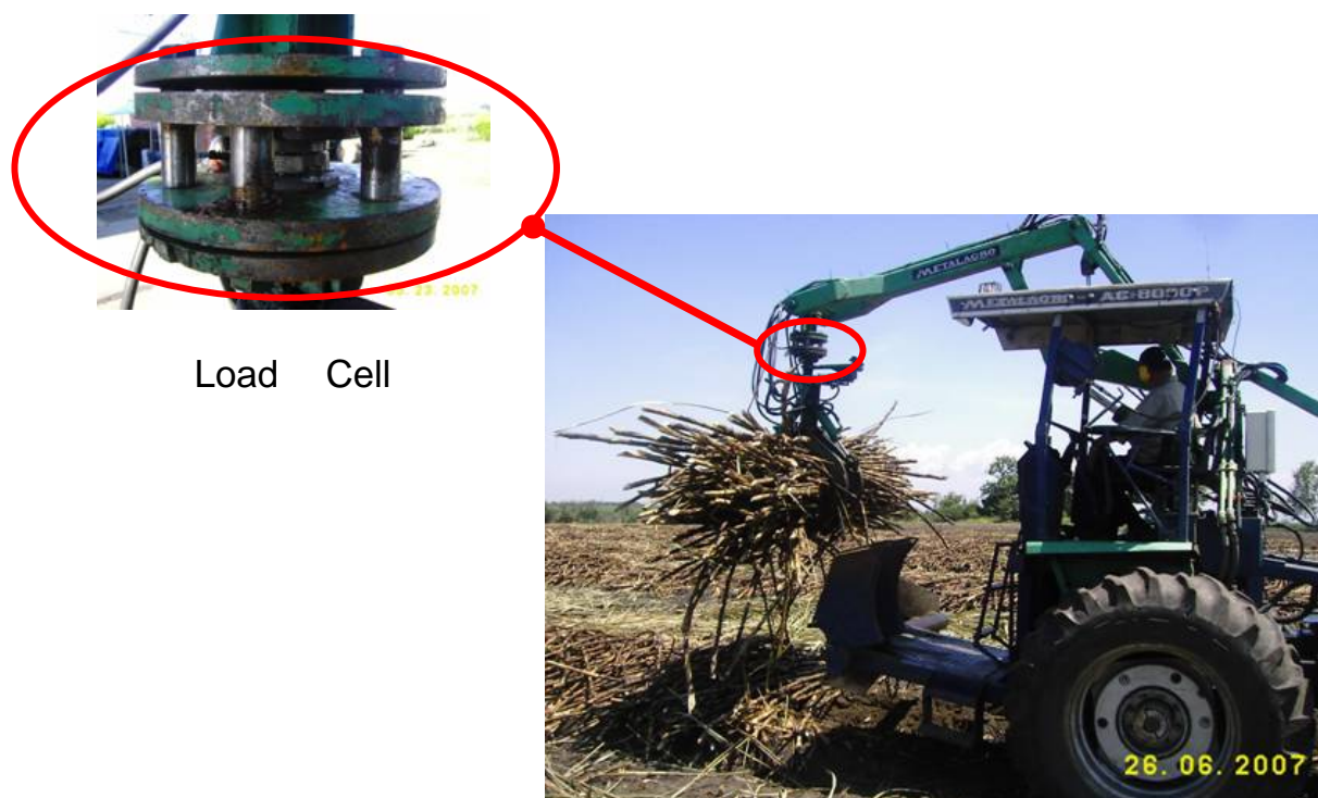
Fig. 1—Mechanical load cell mounting system installed on the cane loader.
