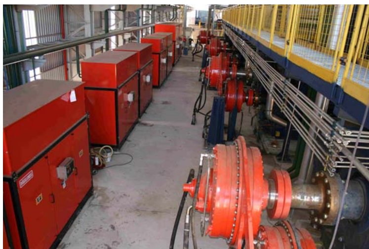
Fig. 2—Santa Isabel milling tandem with individual drives.
