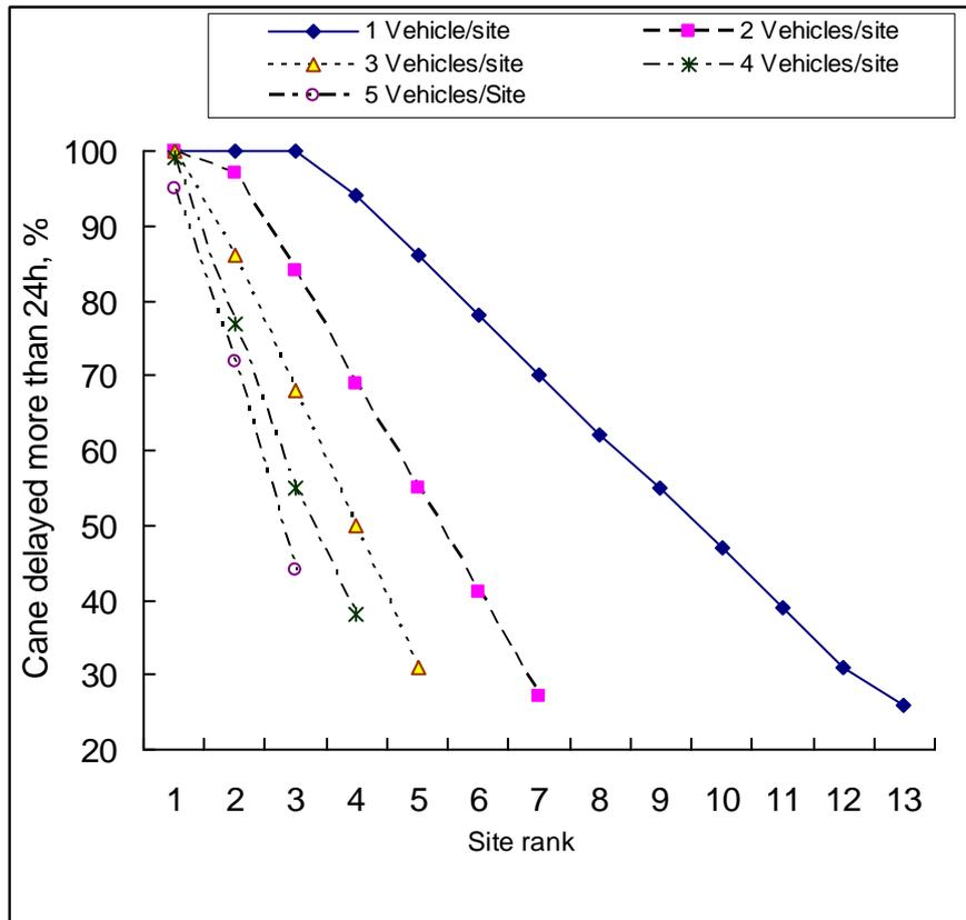
Fig. 3—Percent of vehicle loads delayed more than 24 h to maintain continuous loader operation.
