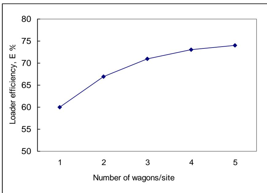
Fig. 2—Loader efficiency as related to combining several vehicles in one site.
