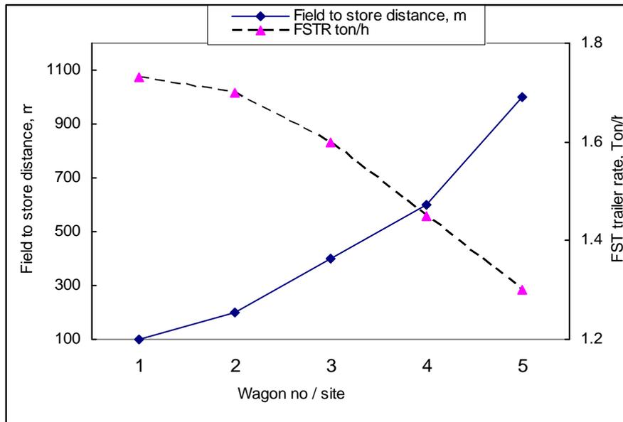
Fig. 1—Effect of combining vehicles in one site as a procedure for improved loader efficiency.
