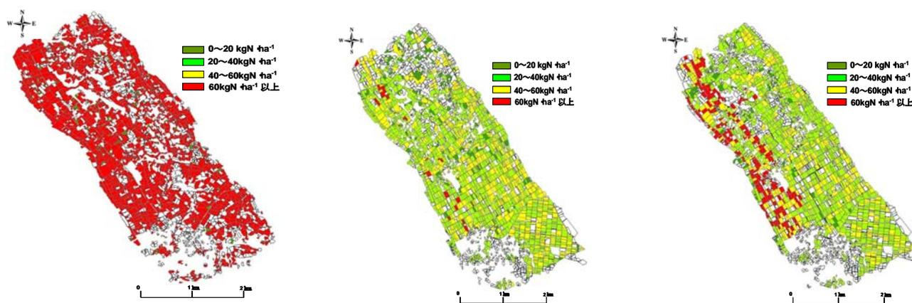
Fig. 2—Nitrate nitrogen loads at Sunagawa groundwater-basin in 1977, 1994 and 2005, respectively (Fujie Rie *et al.*, 2008)
