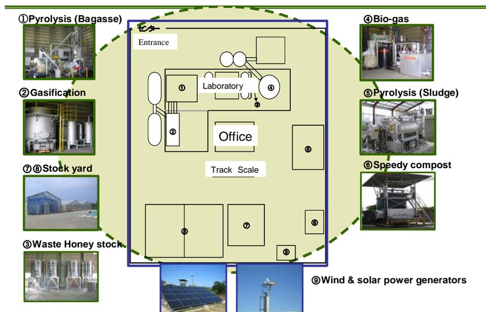
Fig. 1—Biomass refinery systems on Miyako Island, Japan.
