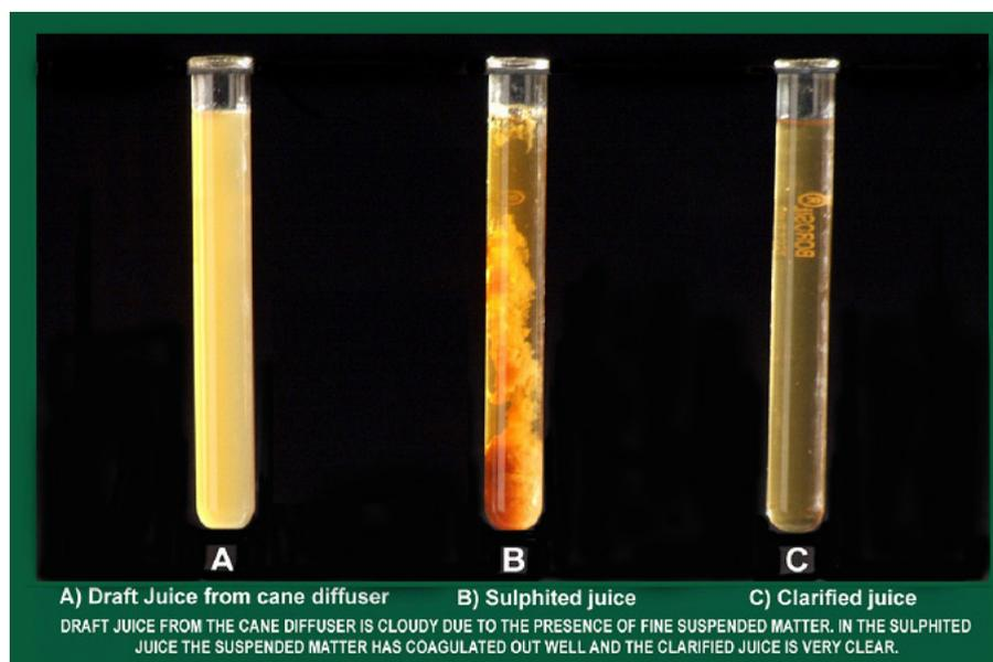
Fig. 3—Colour of draft, sulphited and clarified juice at Taduvali.
