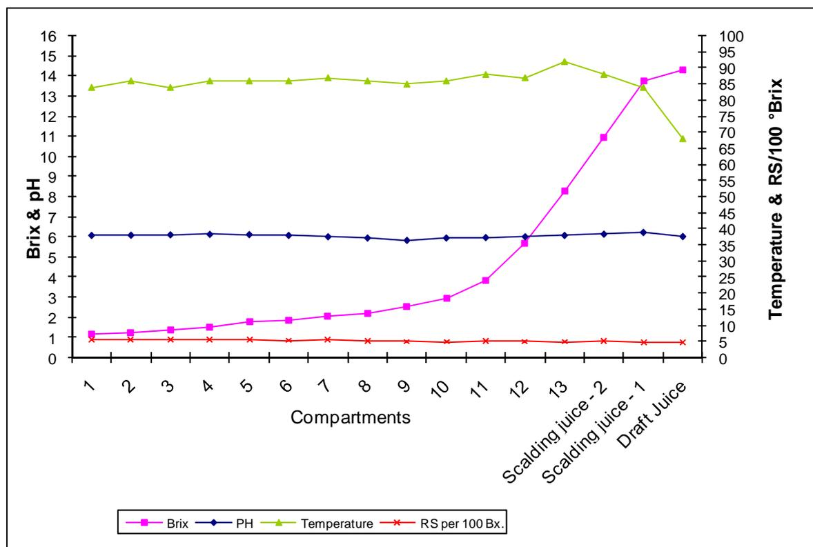
Fig. 2—Graph of concentration (°Brix), pH, Temperature and RS/100°Brix at various compartments of the cane diffuser at Taduvai.
