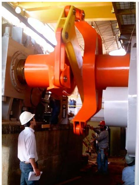
Fig. 3—Rope coupling with link plates fitted with spherical plain bearings.
