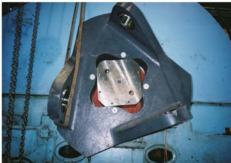
Fig. 7—Hub fitting on shaft.
