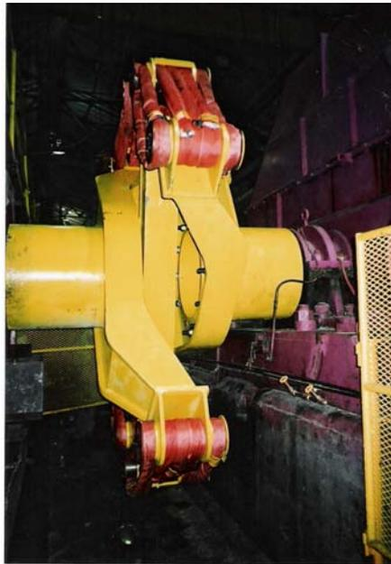
Fig. 2—Rope coupling with polyester slings.
