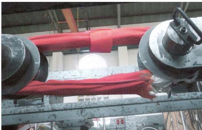
Fig. 4—Polyester sling undergoing destructive test.
