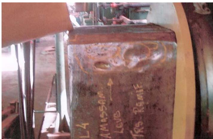
Fig. 5—An un-repaired shaft square.
