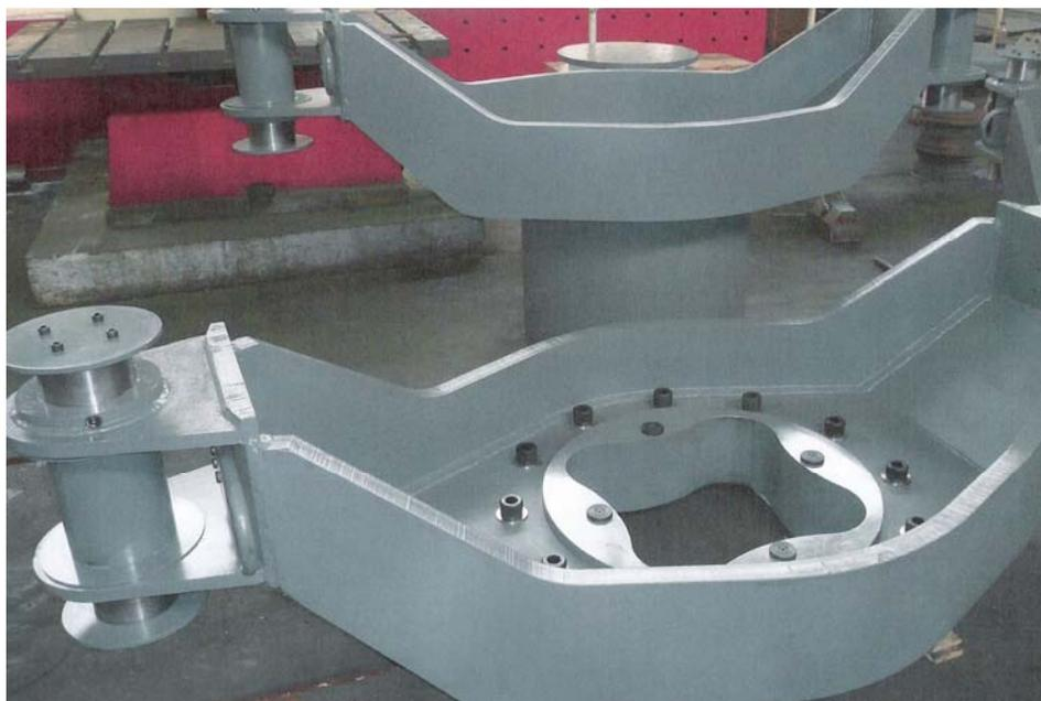
Fig. 9—Yoke-to-Hub connection showing shear pins.
