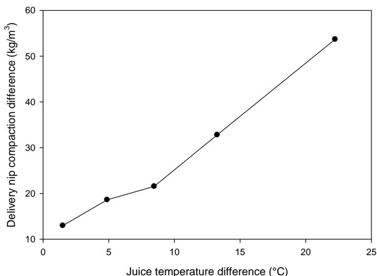
Fig. 3—Increase in delivery nip compaction as a function of the increase in juice temperature for the Macknade tests.
