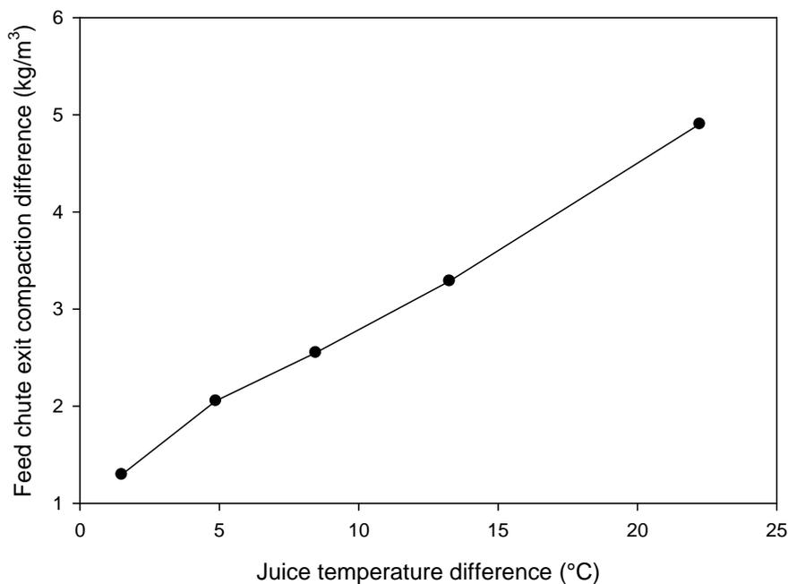
Fig. 5—Increase in feed chute exit compaction as a function of the increase in juice temperature for the Macknade tests.
