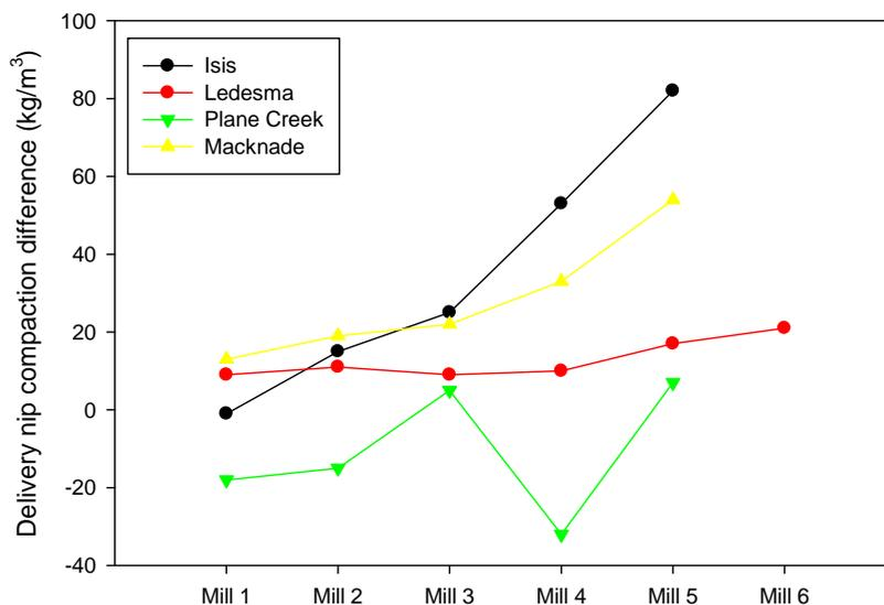
Fig. 2—Increase in delivery nip compaction from lowest to highest temperature added water.
