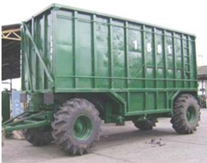
Fig. 5—Prototype of 12 tonne side dumping wagon.
