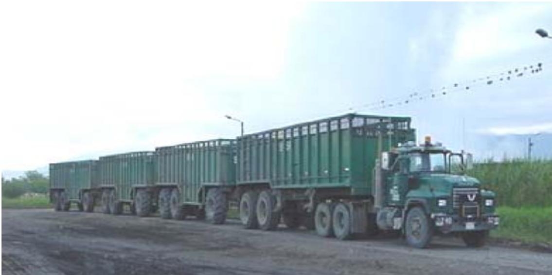
Fig. 1—Typical train composed of four 20 ton wagons.
