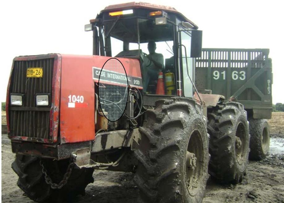
Fig. 8—AIC-888 Instruktor Fuel flow meter, on a 9230 tractor.
