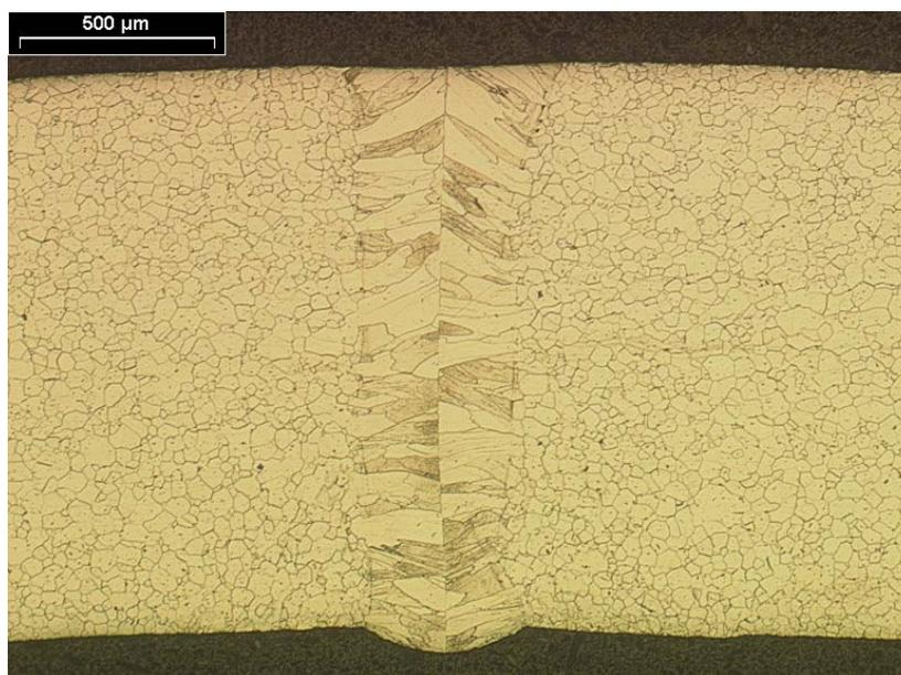
Fig. 2—Micrography of a laser weld.
