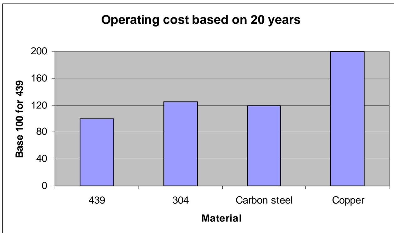
Fig. 4—Calculated operating costs for different materials.
