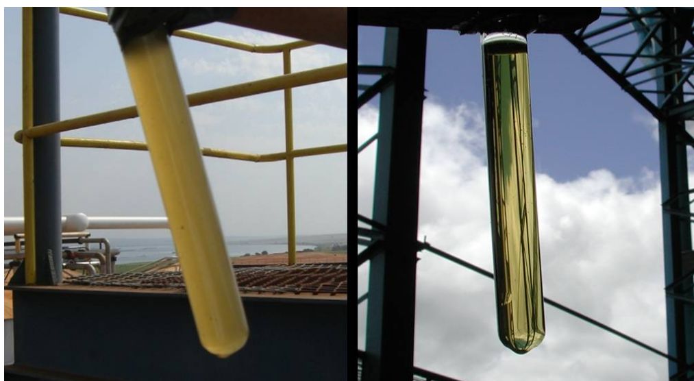
Fig. 1—Samples of turbid clarified juice suitable for fermentation (left) and clear clarified juice suitable for sugar production (right).
