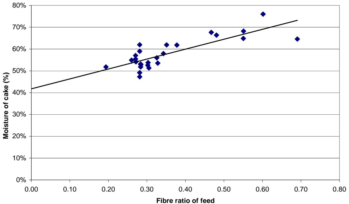
Fig. 4—Effect of the fibre ratio in the mud feed on final product moisture when mud is processed through a centrifuge.
