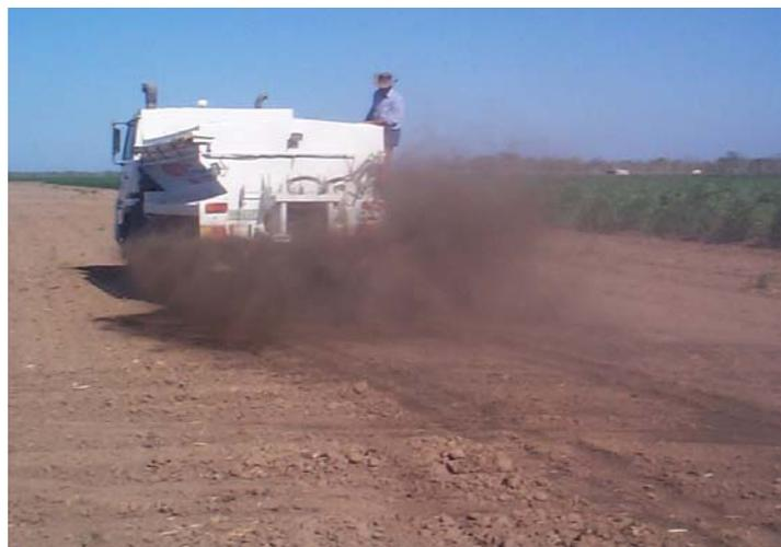
Fig. 5—Spreading centrifuge mud using a truck set up to spread fertiliser and gypsum.
