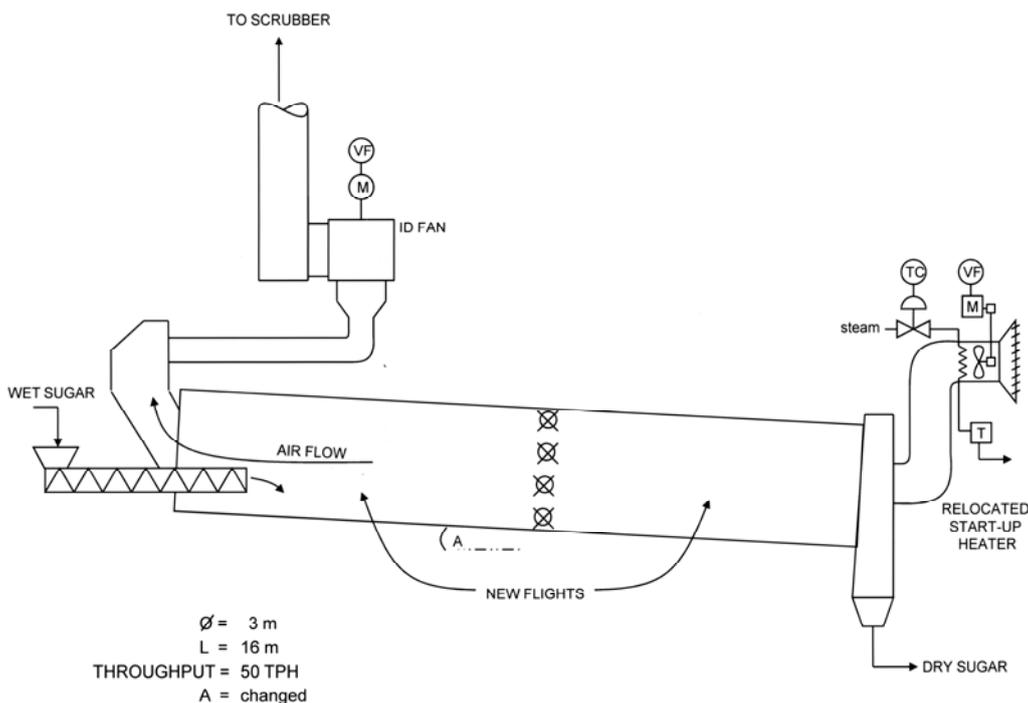
Fig. 2—Sugar dryer after conversion.
