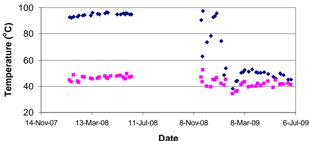
Fig. 6—Inlet air and product sugar temperatures.
