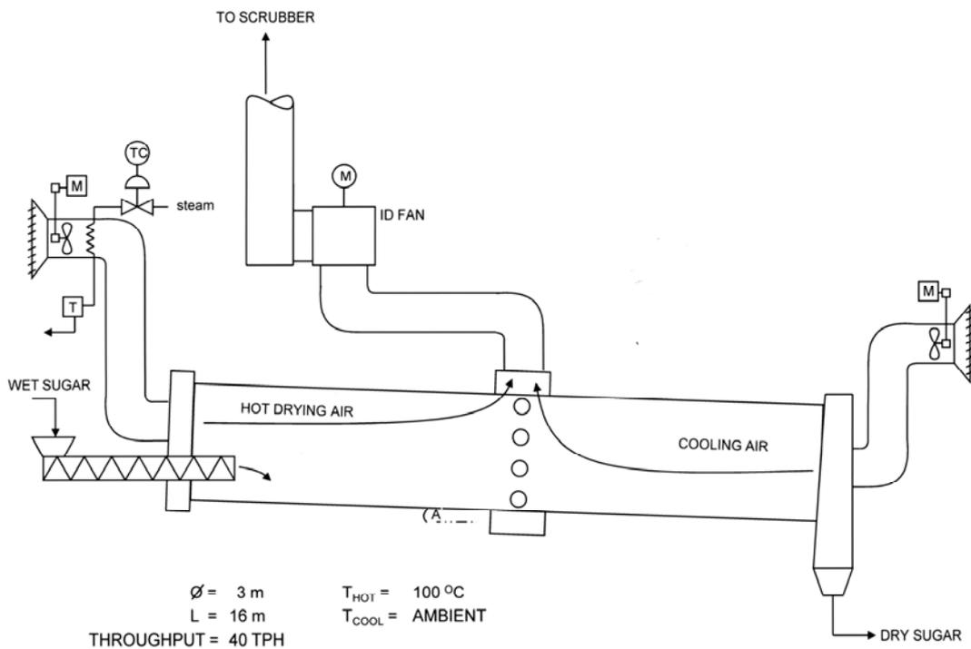
Fig. 1—Sugar dryer before conversion.
