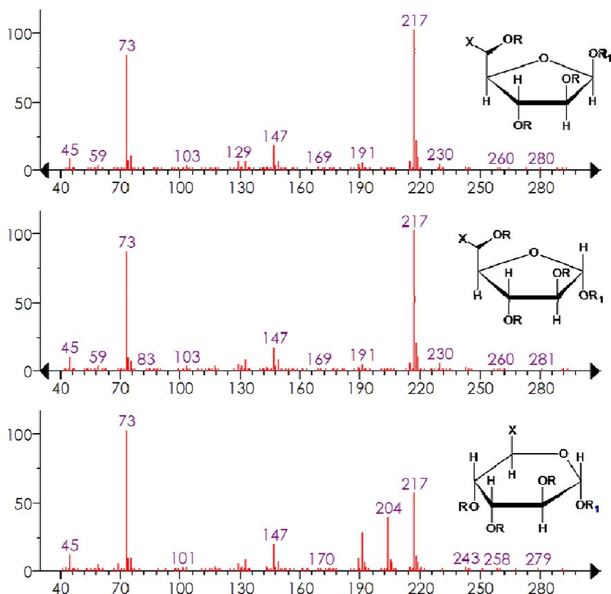
Fig. 5—Comparison of the mass spectra between the  $\beta$ - and  $\alpha$ -furanoside forms (upper and middle spectra) and the  $\alpha$ -pyranoside form (lower spectra) of TMSi derivatised arabinose. (R = R<sub>1</sub> = TMSi; X = H). [y-axis = Abundance, x-axis =  $m/z$ ]
