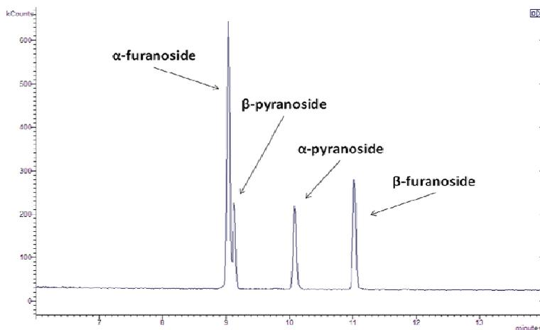
Fig. 4—GC chromatogram showing separation of TMSi arabinose derivatives showing  $\alpha$ - and  $\beta$ - anomers of the pyranoside and furanoside forms.
