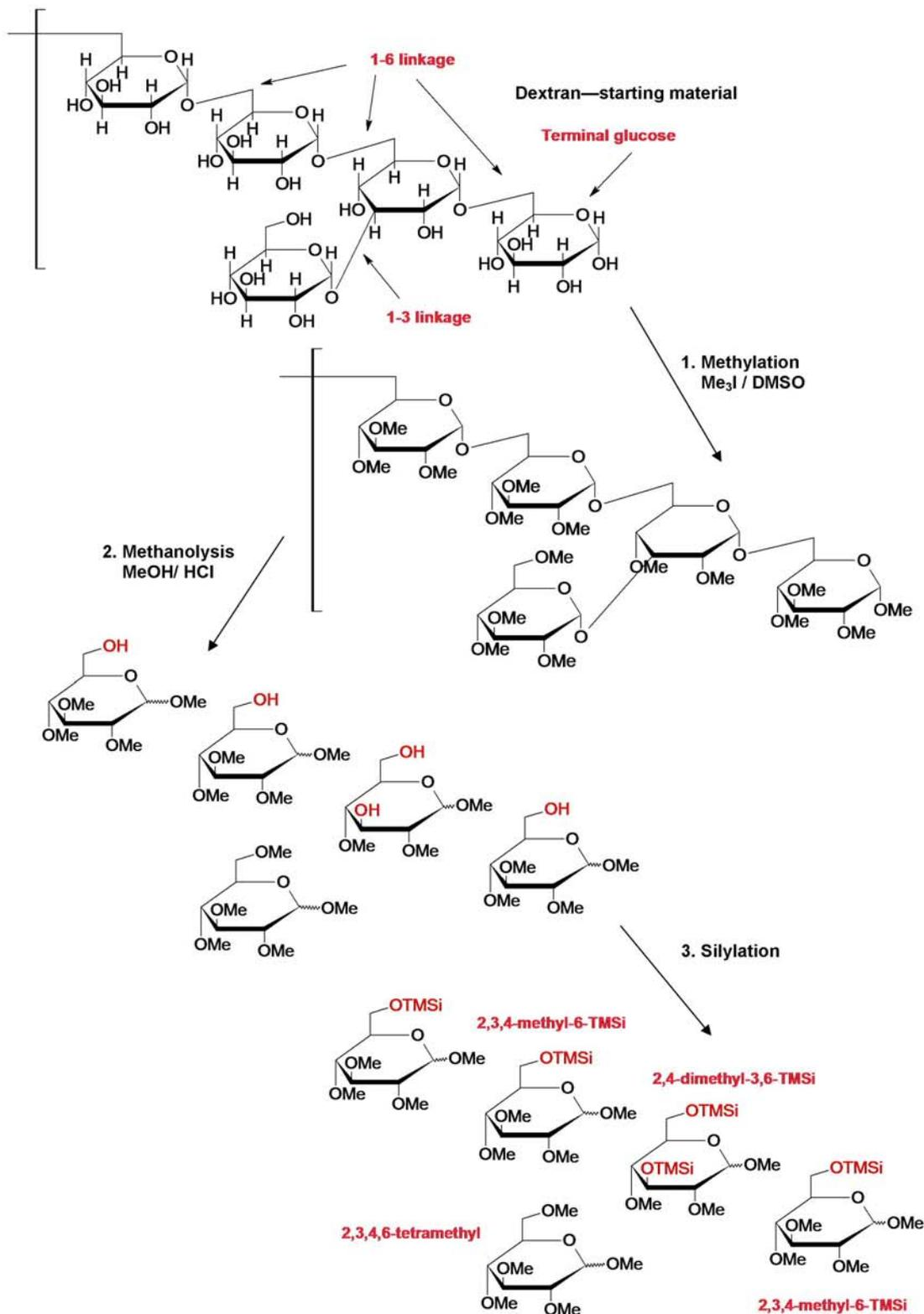
Fig.9—Diagram showing the method of structural analysis using dextran as a model compound. The steps include methylation (Step 1), methanolysis (Step 2) and silylation (Step 3) to produce methylated, TMSi derivatives dependent on the position in the polymer
