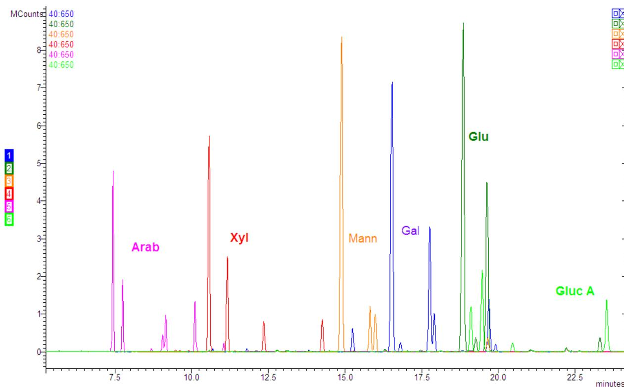
Fig. 6—Chromatogram showing the separation of a mixture of TMSi sugars. Arab = arabinose; Xyl = xylose; Mann = mannose; Gal = galactose; Glu = glucose; Gluc A = gluconic acid.
