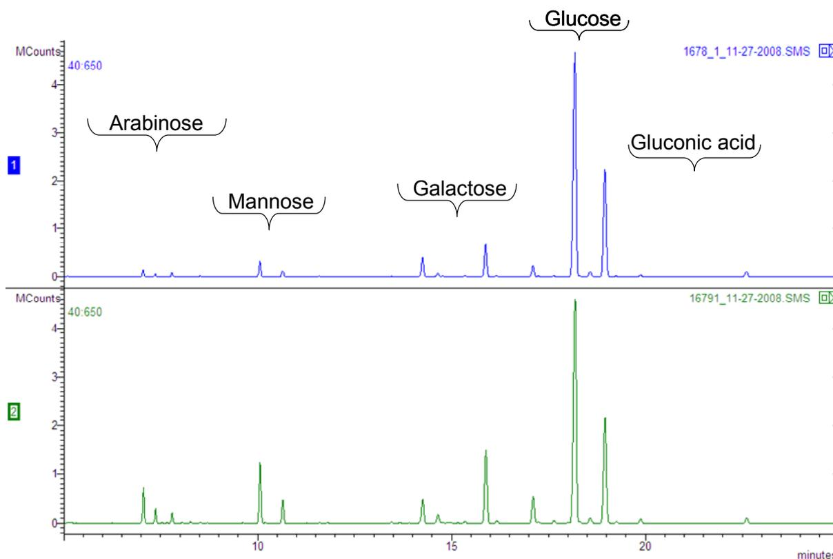
Fig. 11—Chromatograms comparing a normal (upper) and 'hard-to-boil' massecuite (lower).
