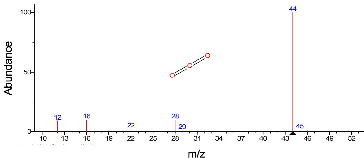
Fig. 2—Mass spectrum of carbon dioxide.
