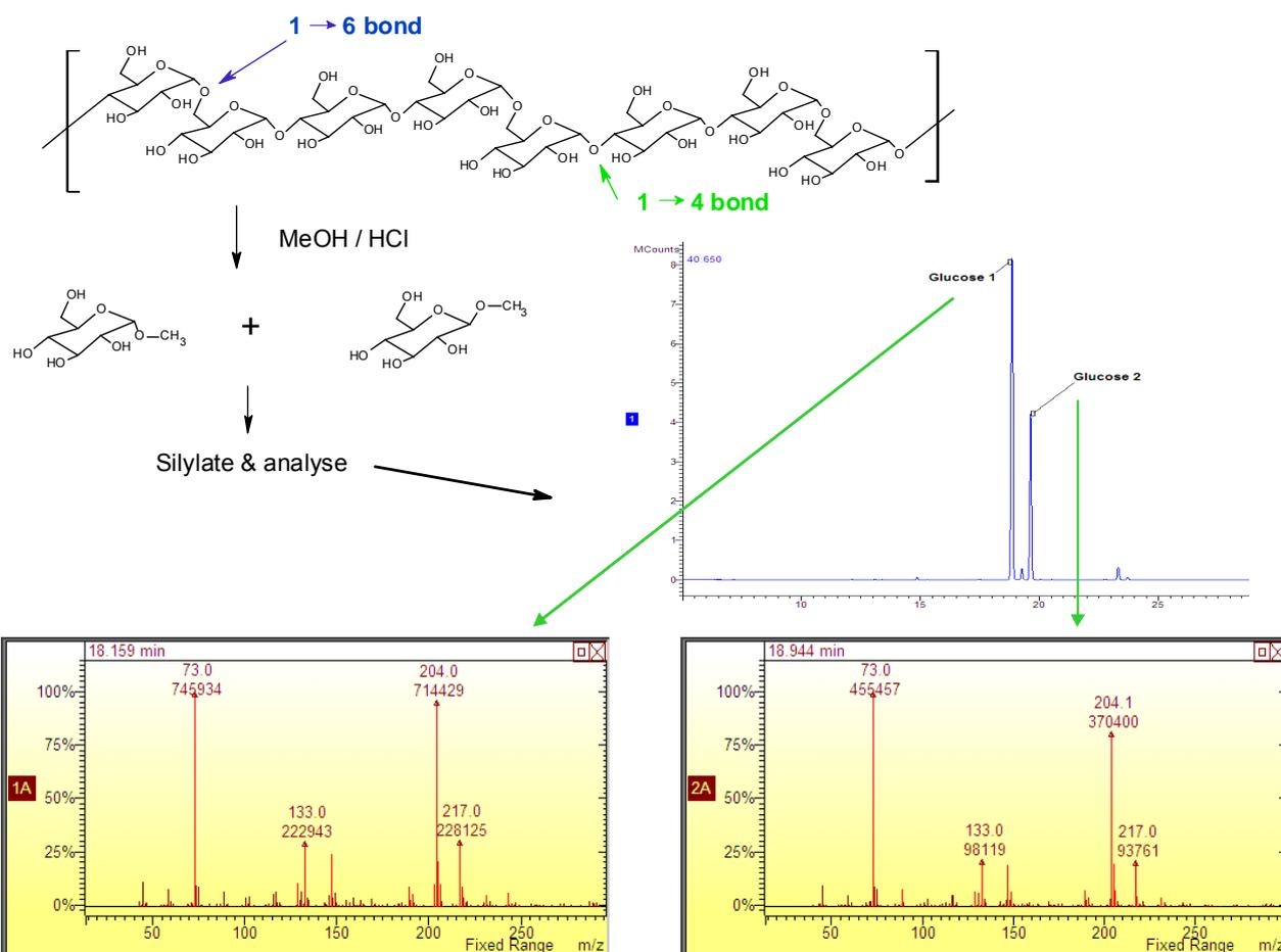
Fig. 7—Methanolysis of pullulan showing hydrolysis and methylation at position 1 and resultant chromatogram after silylation showing only pyranoside glucose peaks.
