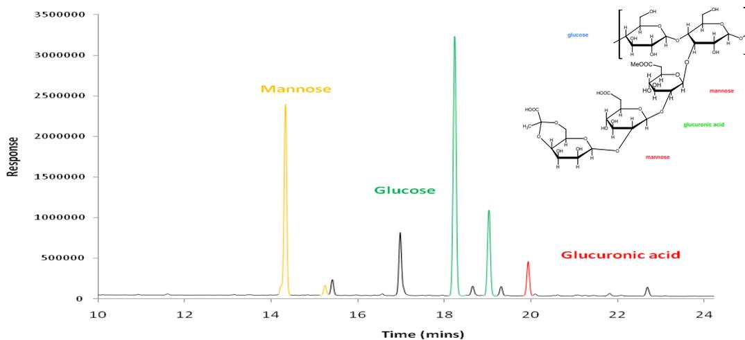
Fig. 8—Chromatogram from the methanolysis of xanthan gum showing the compositional sugars – glucose, mannose and glucuronic acid.
