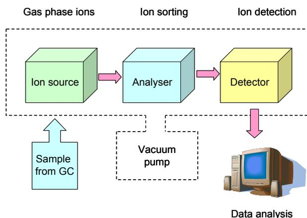
Fig. 1—Diagram of a GC mass spectrometer.
