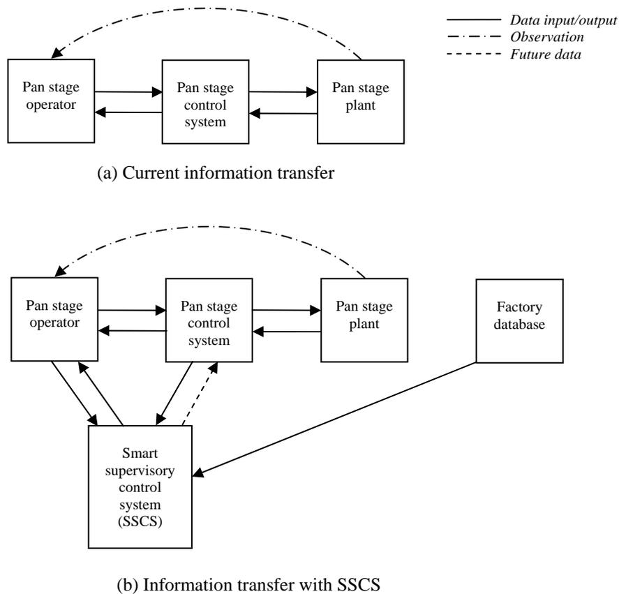
Fig. 2—Information transfer for current pan stage control and with the SSCS.
