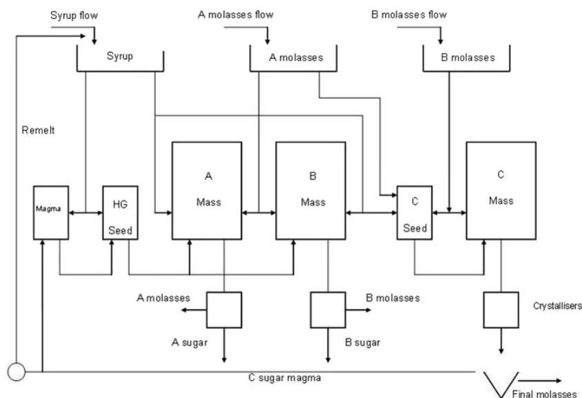
Fig. 1—Flowscheme for the pan stage operations in Australian sugar factories.
