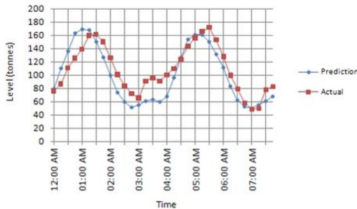
Fig. 1—Comparison of forward prediction of A molasses stock tank levels with actual data.
