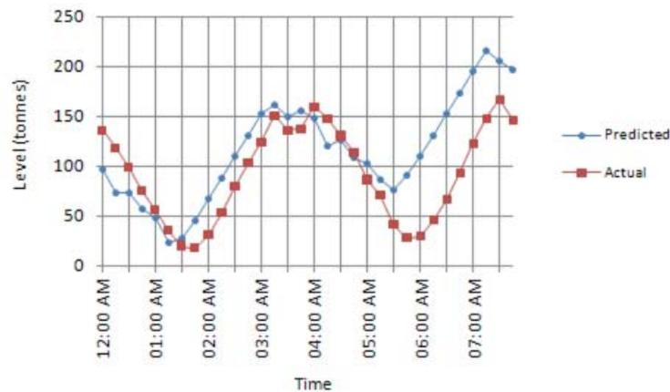
Fig.4—Comparison of forward prediction of syrup stock tank levels with actual data.
