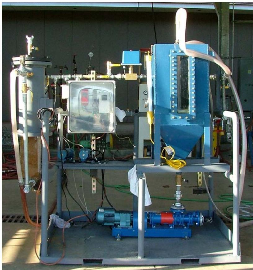
Fig. 1—Pilot clarification module tested at Raceland (2007 campaign).
