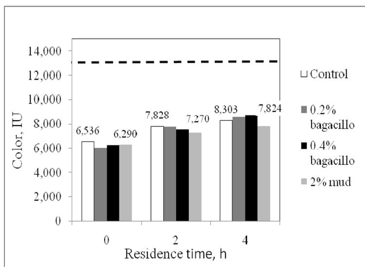
Fig. 6—Colour of raw juice (13 200 IU), juice clarified by hot liming (control), and juice clarified by hot liming after additions of bagacillo or dry mud to the raw juice.
