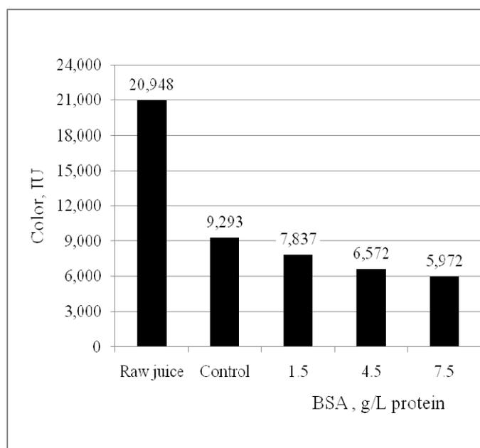
Fig. 5—Colour of raw juice, clarified juice by hot liming (control), and clarified juice after sequential additions of bovine serum albumin.
