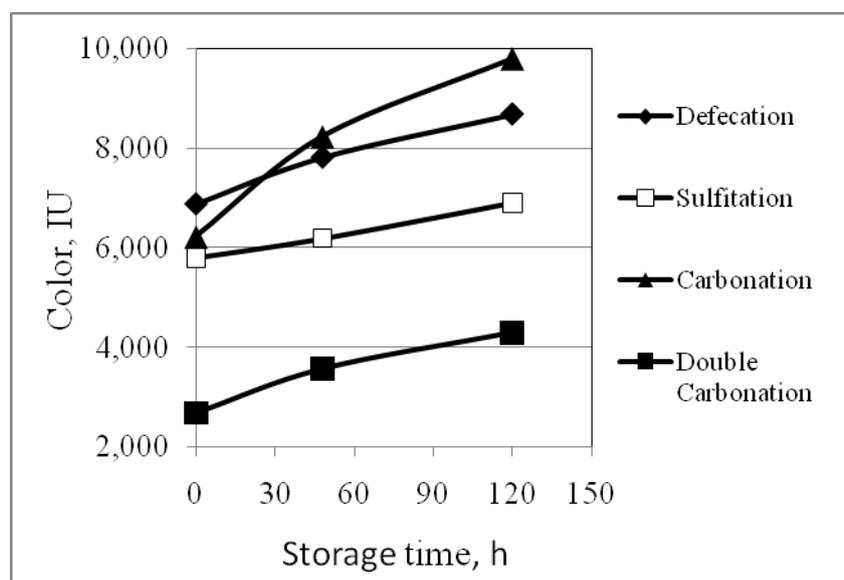
Fig. 2—Colour increase of 60 – 70 brix syrup produced from the four different clarification procedures and stored at 70°C.
