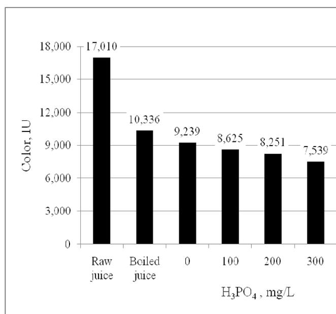
Fig. 4—Colour of raw juice, raw juice after boiling and clarified juice by hot liming after addition of phosphoric acid.
