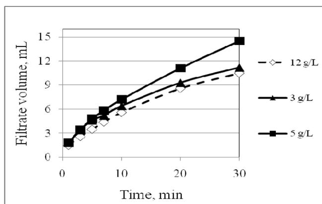
Fig. 7—Filterability of thickened mud from the modified process (solid lines) with 3 and 5 g/L of CaO, and that of the industrial double carbonation process with 12 g/L CaO (dotted line).
