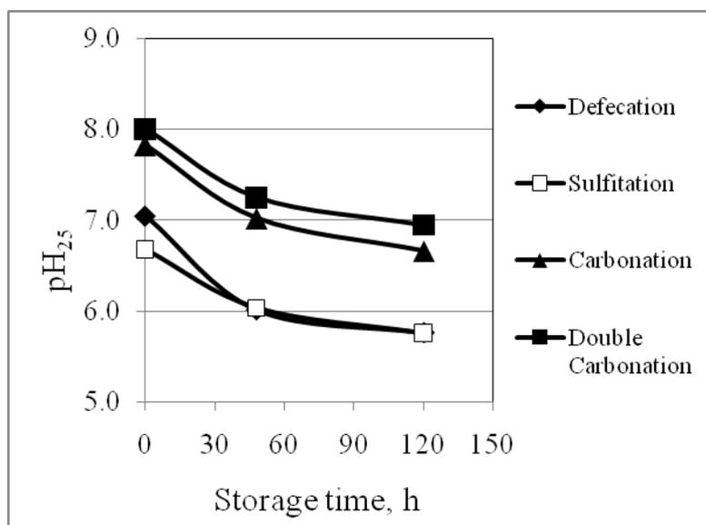
Fig. 3—pH drop during storage of syrup produced by the four different clarification procedures.
