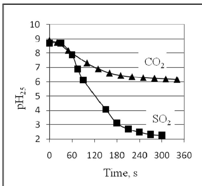
Fig. 1—Absorption rate of carbon dioxide and sulfur dioxide in limed juice.
