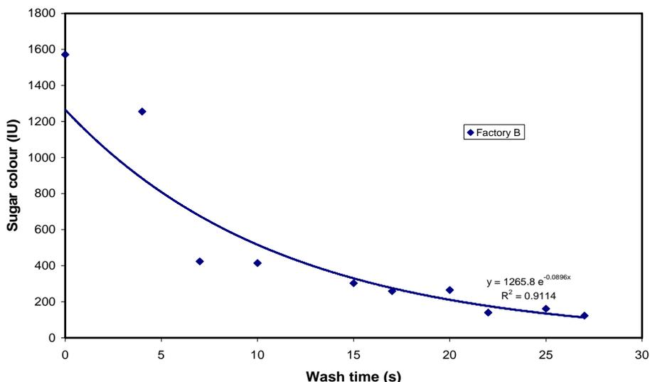
Fig. 2—Final sugar colour as a function of wash water time for factory B. (Western States centrifugal, 54 x 40, 480 kPag, 85–95°C).
