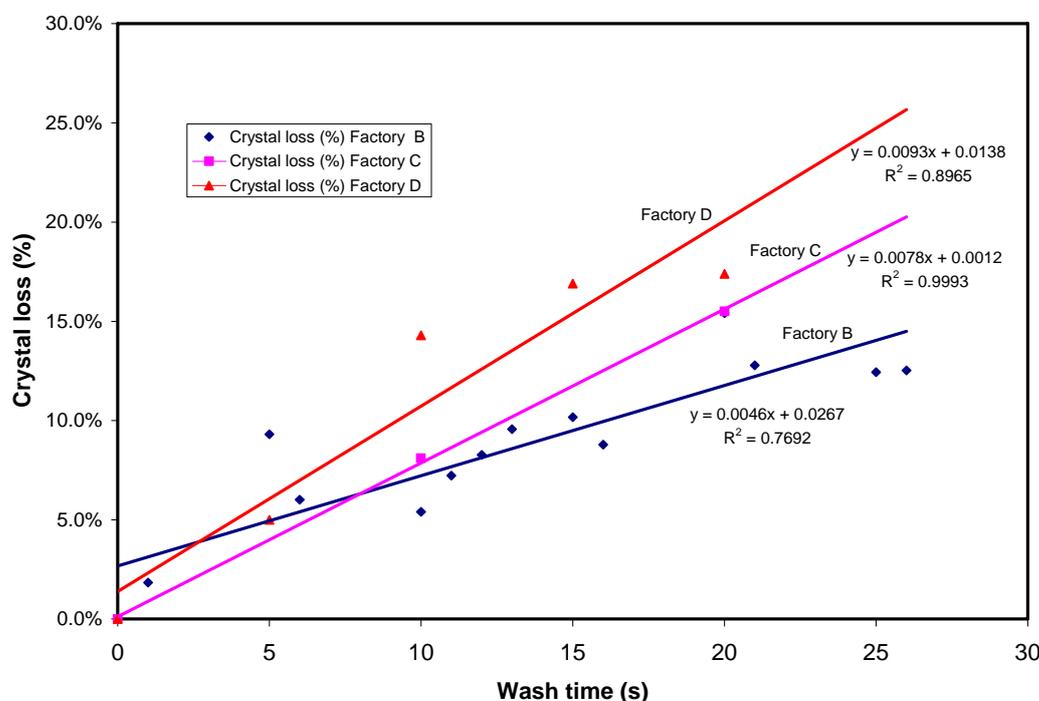
Fig. 1—Crystal loss as a function of wash time for three factories.
