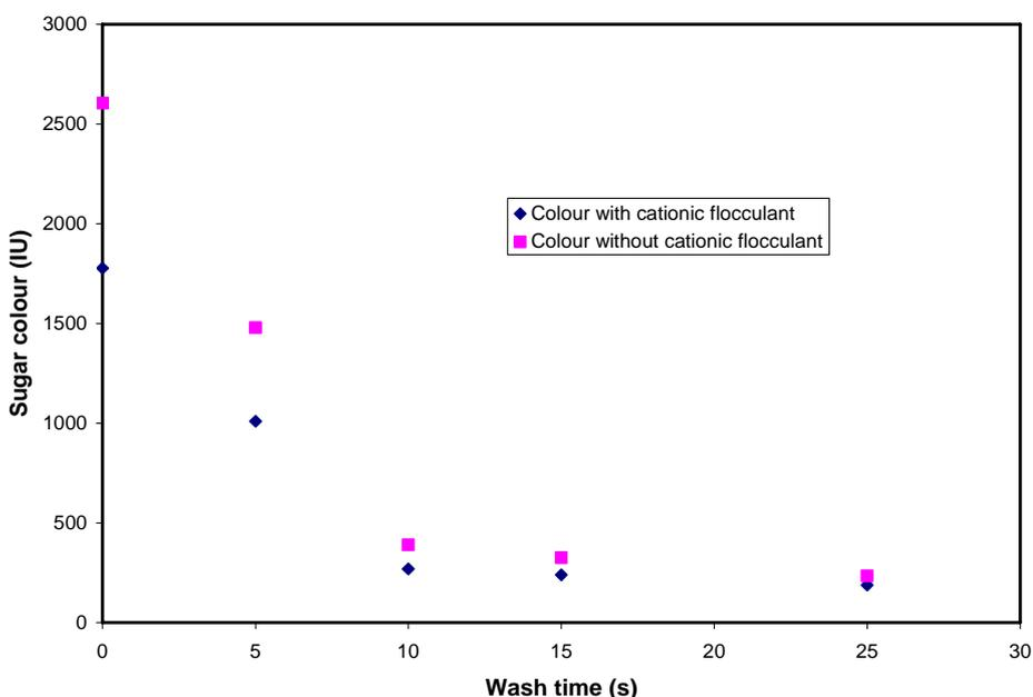
Fig. 3—Final sugar colour as a function of wash water time for factory C (Western States centrifugal, 48x36, 550 kPag, 80–90°C).
