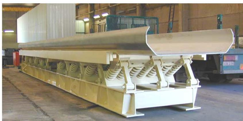
Fig. 3—Example of a vibratory conveyor.
