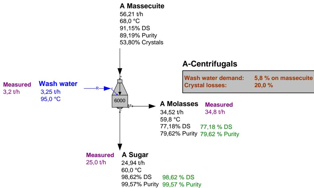
Fig. 3—Simulation of an A centrifugal station.
