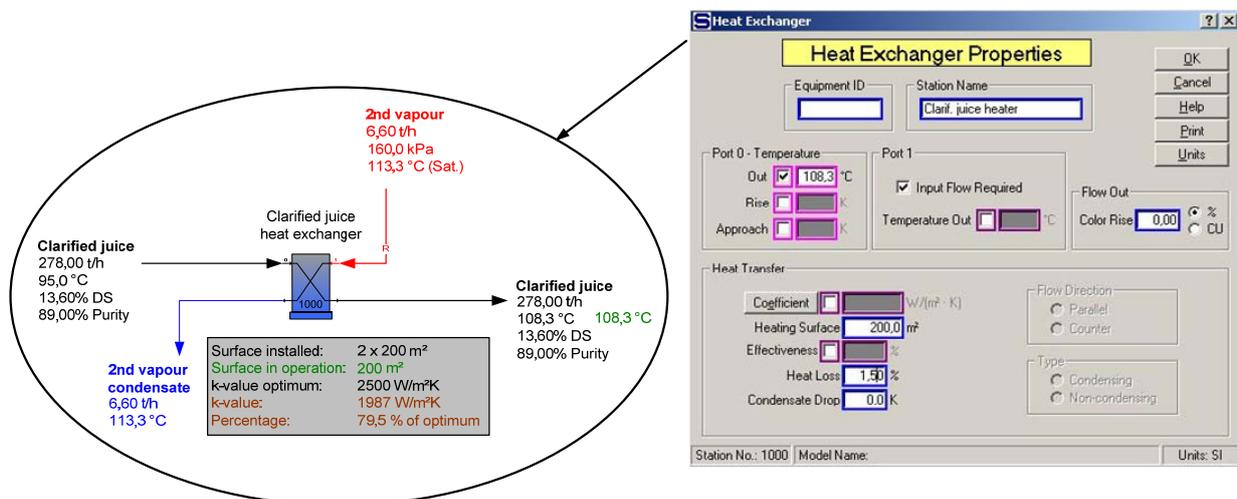
Fig. 1—Heat exchanger with open model property window.
