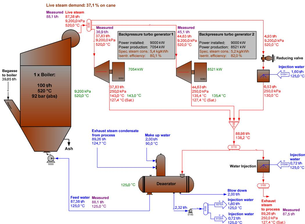
Fig. 4—Power station simulation.
