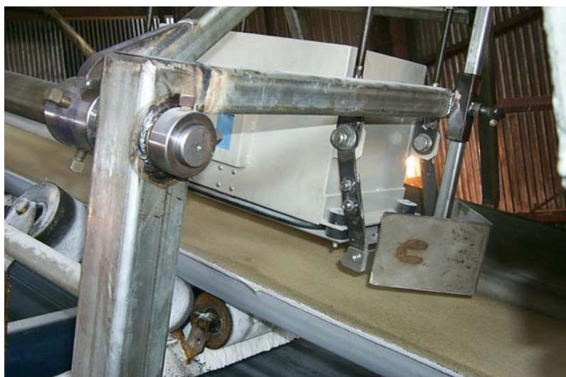
Fig. 1—Typical mounting system for the SAS scanning head over a sugar conveyor belt.
