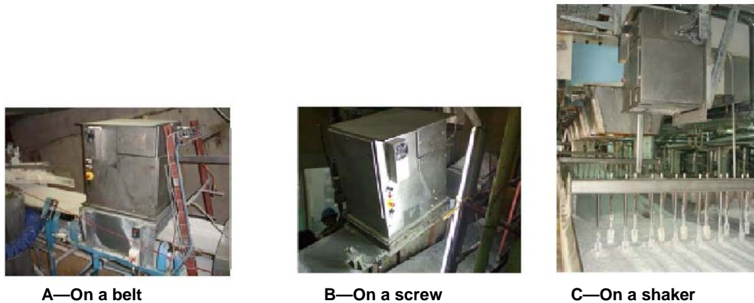
Fig. 1—Illustrations of the Colobserver® installed on different conveyor systems.
